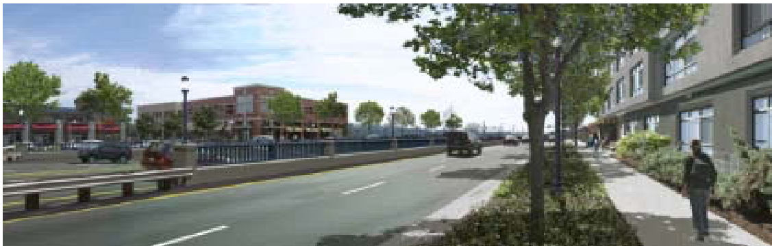
Visualization of US-29 facing south towards Hydraulic Road intersection, India Road at left, Albemarle Place development at right. Recommended Option of grade-separated intersection (SPUI) with US-29 through lanes passing under Hydraulic
