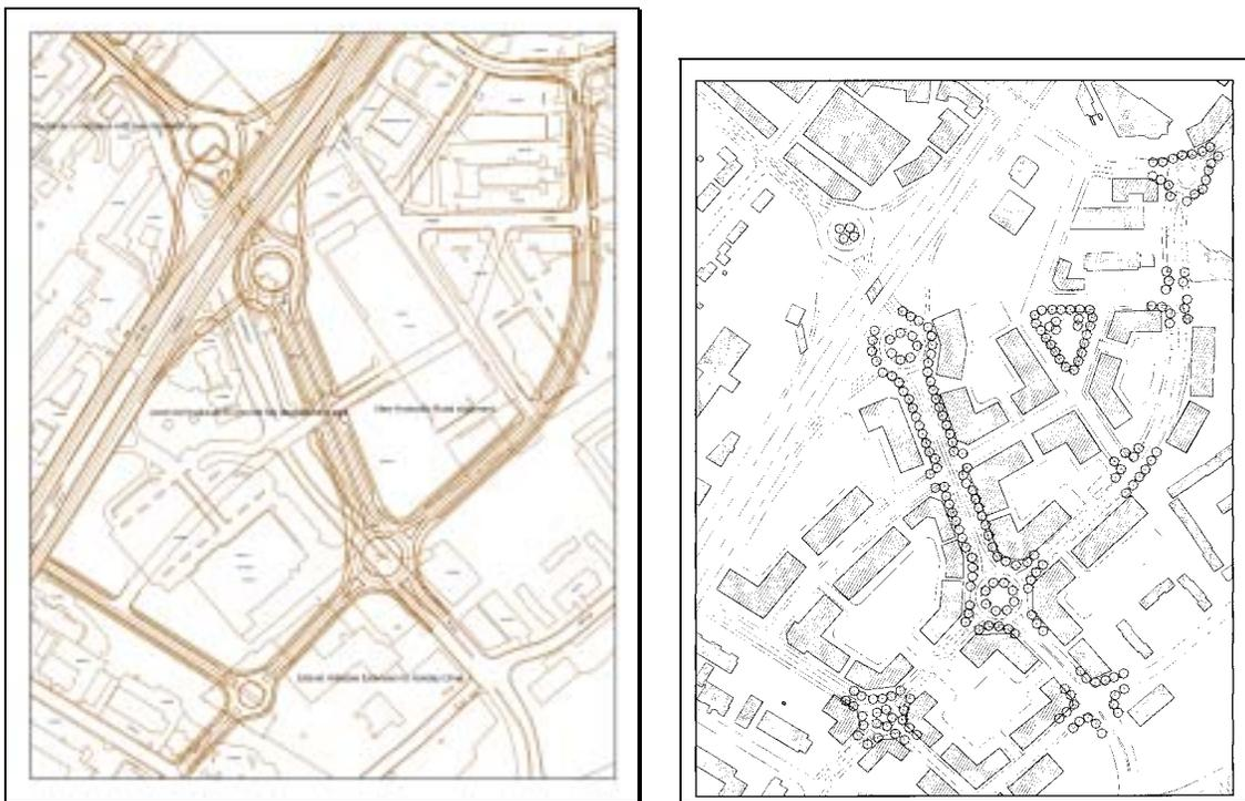
*Figure 37 Diagram at left shows realignment of Hydraulic with underpass just north of existing Hydraulic to allow for traffic flow during construction. Diagram at right shows eventual redevelopment of the area around the new road system.*
