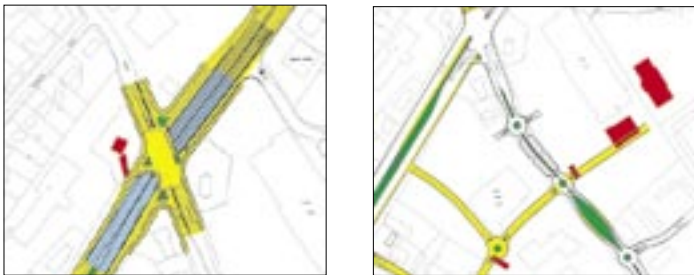
Redesign of Hydraulic Road/ US29 into a SPUI (left); Redesign of Hydraulic Road with roundabouts and medians (right)
