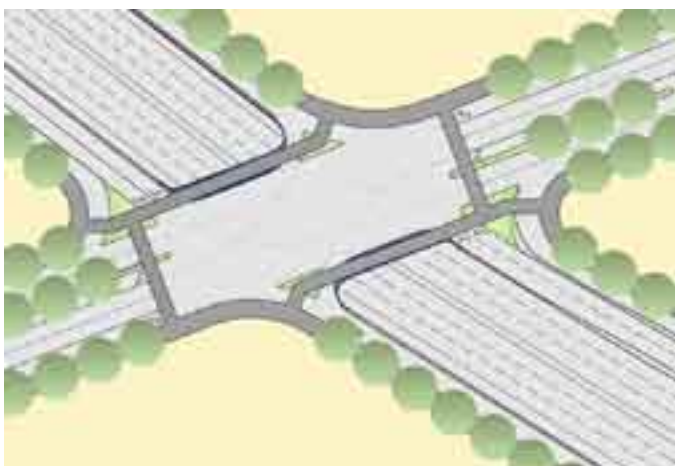
The SPUI configuration requires careful design to create high-quality pedestrian and bicycle access
