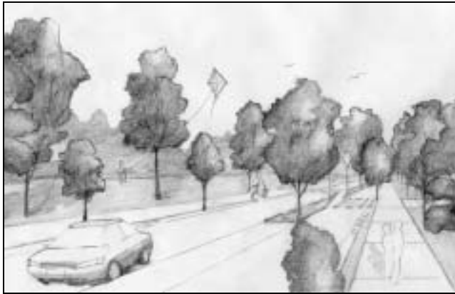
Pleasant pedestrian environment enhanced with landscaped median crosswalk islands.
